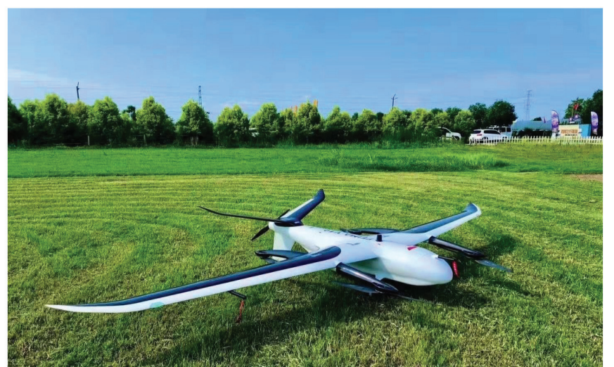
Figure 2. Pegasus V10 large-load vertical takeoff and landing UAV.
