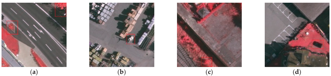
Figure 4. Example of a small object in a complex scene of an HR remote sensing image. The red box selected is the small object that is easy to be ignored. Vegetation in (a). Cars in (b). Vegetation in (c). Cars in (d).
