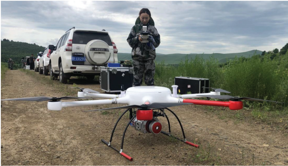
Figure 4. Hurtigruten six-rotor UAV Long-120 equipped with the Hurtigruten ARS-1000 L long-range LiDAR measurement system.
