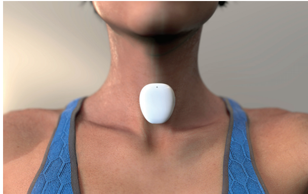
Figure 1. The placement of the Clebre audio and motion sensor.
