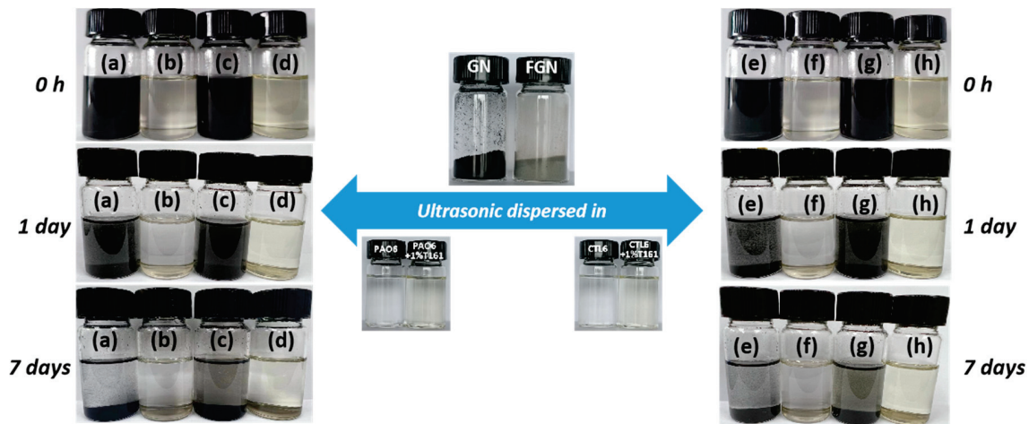
Figure 5. Images of dispersion oils with 100 ppm of graphene additives over time: (a) GN, (b) FGN, (c) GN-1%T161, and (d) FGN-1%T161 in PAO6; (e) GN, (f) FGN, (g) GN-1%T161, and (h) FGN-1%T161 in CTL6.
