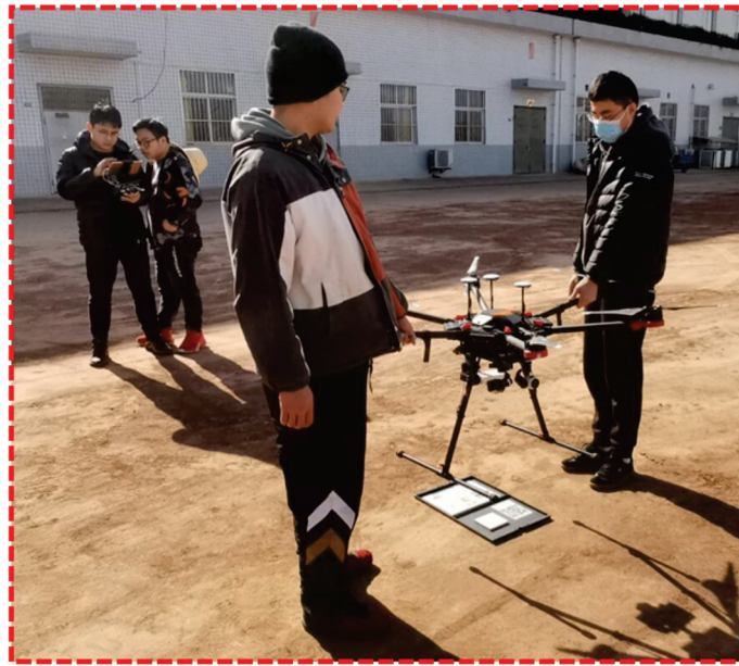
Figure 5. Multispectral camera radiometric calibration.
