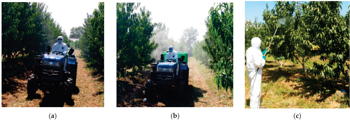
Figure 2. Photos of the sprayers in the peach orchard during the experiment. (a) Trailer air-assisted orchard sprayer, (b) mounted air-assisted orchard sprayer, (c) orchard spray gun.
