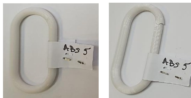
Figure 9. The appearance of a chain link made of ABS polymer material before (left) and after (right) breaking, respectively.
