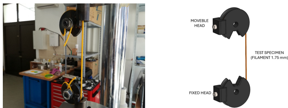
Figure 4. Uniaxial tensile testing of filament procedure: (left) equipment for uniaxial filament testing and (right) sketch of equipment.
