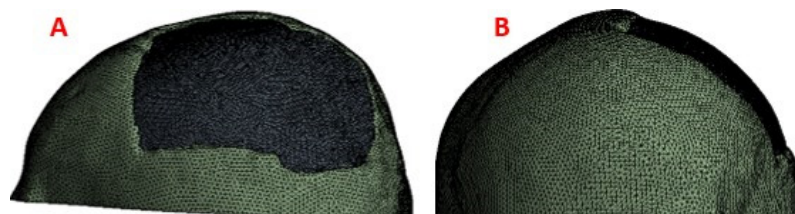
Figure 7. Mesh elements: (A) Mesh of the implant with fixation towards the skull; (B) The meshing of the cranial model with the implant.
