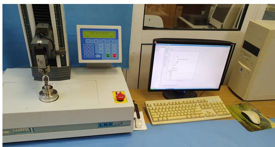
Figure 6. Components of equipment used for tensile testing of chain links.
