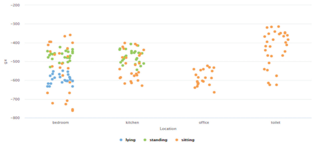
Figure 23. Analysis of the gyroscope data (in the X-direction) for different behavioral patterns associated with different ADLs performed in the given simulated smart home environment.
