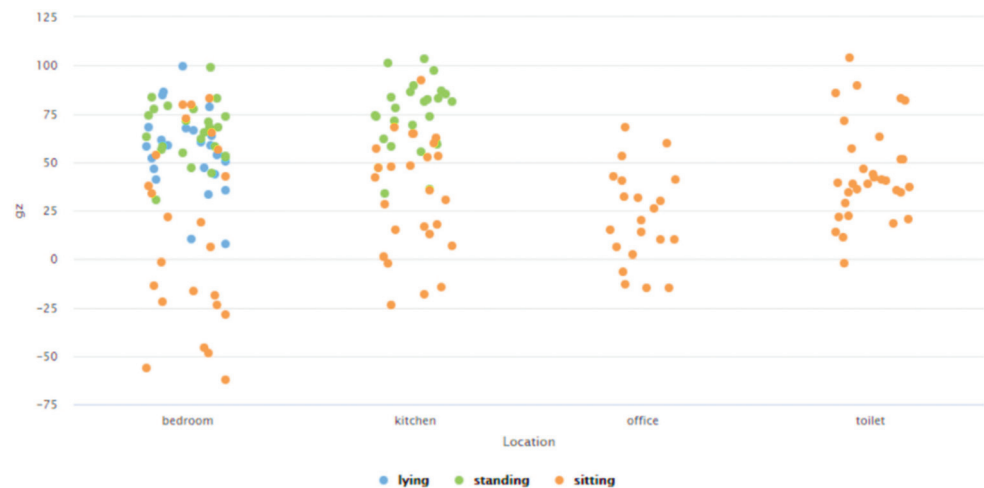
Figure 25. Analysis of the gyroscope data (in the Z-direction) for different behavioral patterns associated with different ADLs performed in the given smart home environment.
