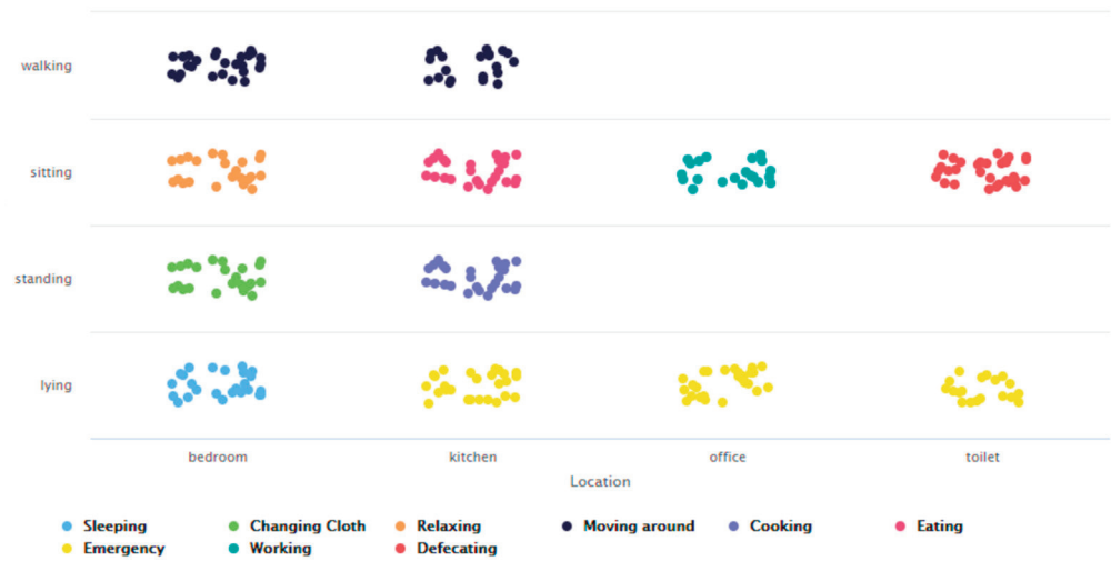
Figure 4. Representation of common and distinct behavioral patterns associated with the different ADLs performed in the different spatial locations or ‘zones’ in a given IoT-based environment.
