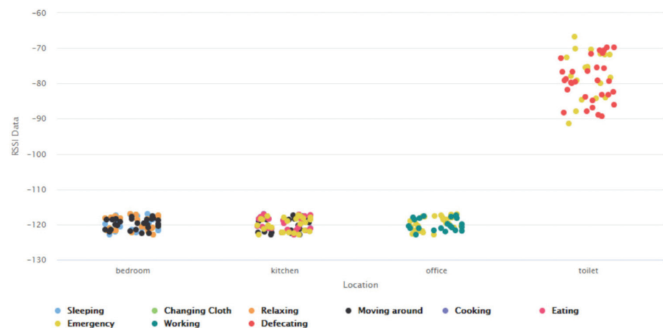
Figure 16. Analysis of RSSI data coming from different BLE scanners and BLE beacons when different activities were performed in the toilet.
