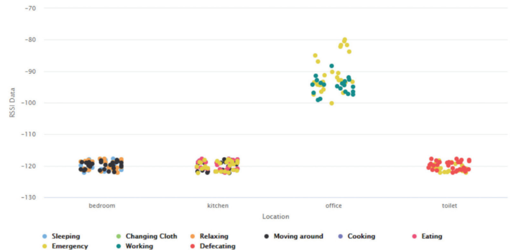
Figure 15. Analysis of RSSI data coming from different BLE scanners and BLE beacons when different activities were performed in the office area.
