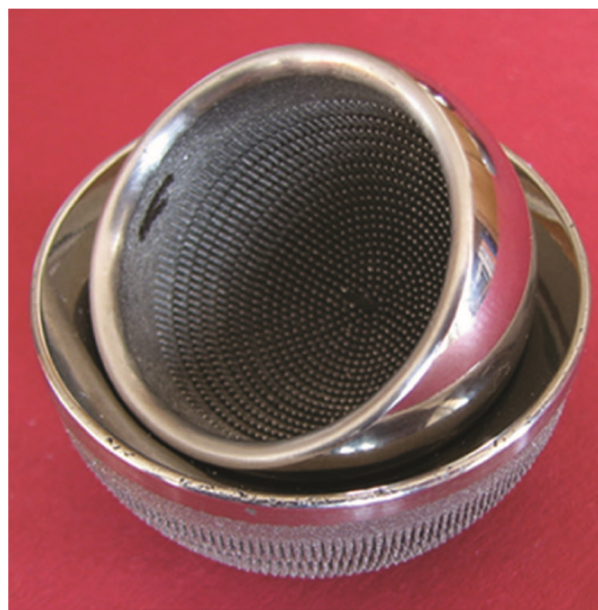
Figure 3. Prototype of hip resurfacing arthroplasty endoprosthesis with the multi-spiked connecting scaffold (MSC-Scaffold) [149].
