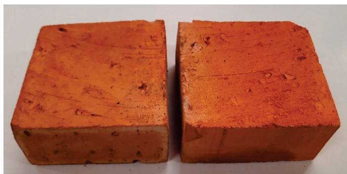
Figure 1. A brick sample used for tests.
