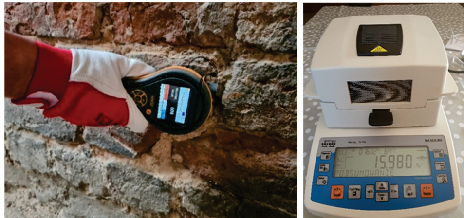
Figure 8. Assessment of the moisture level of walls using the radio and laboratory dry-oven test method (photos by the authors).
