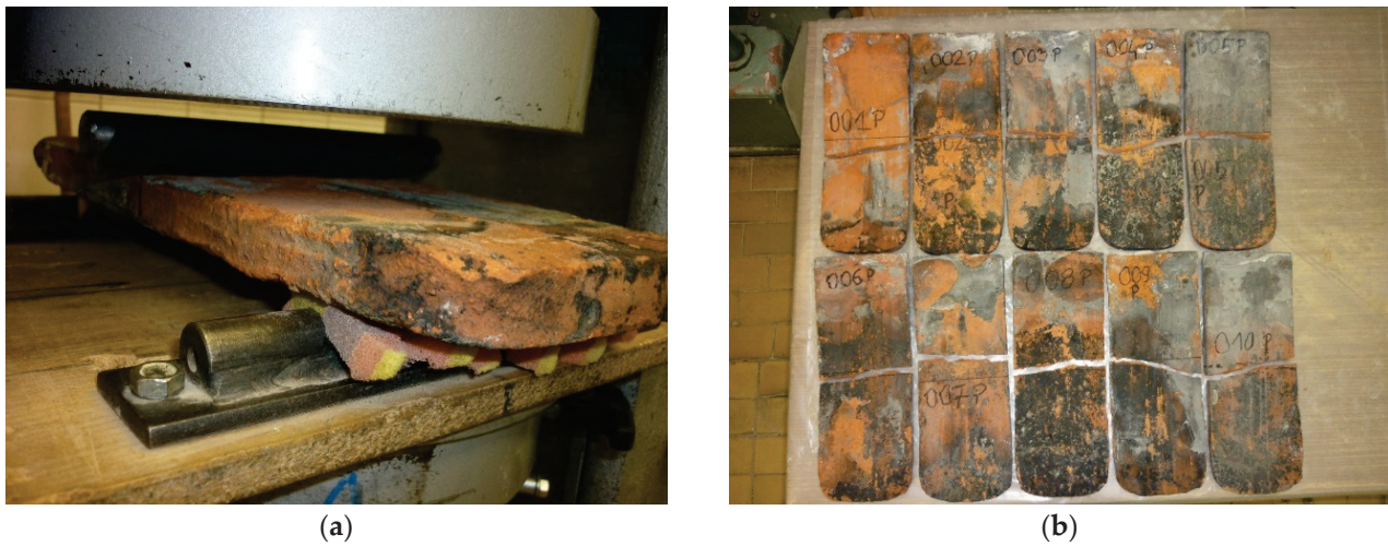
Figure 11. Flexural load capacity test: (a) tile in the testing machine during flexural capacity tests; (b) tiles (Nos. 001–010) after flexural strength tests.
