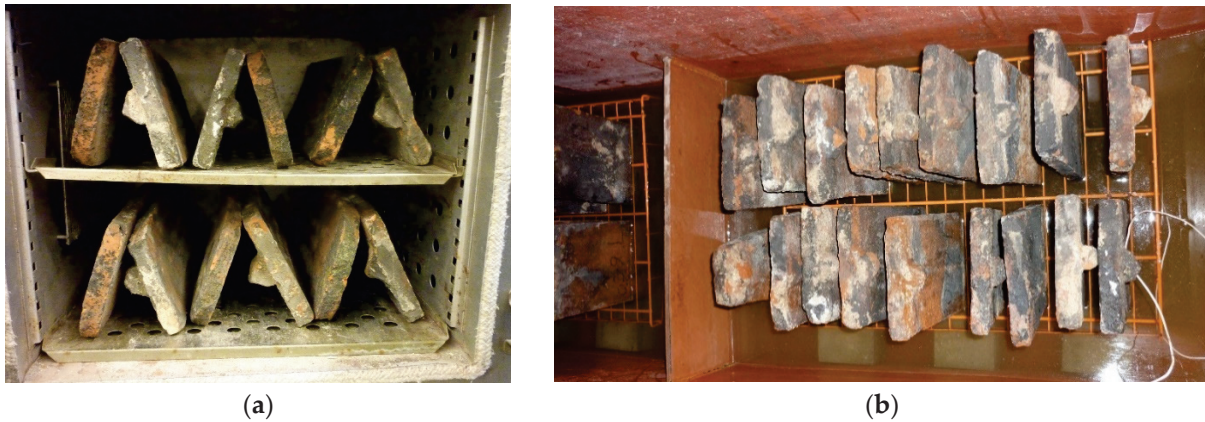
Figure 5. Absorption test: (a) drying of tiles to constant weight at a temperature of 110\text{ °C} \pm 5\text{ °C} ; (b) roof tiles in a chamber with 100% humidity.
