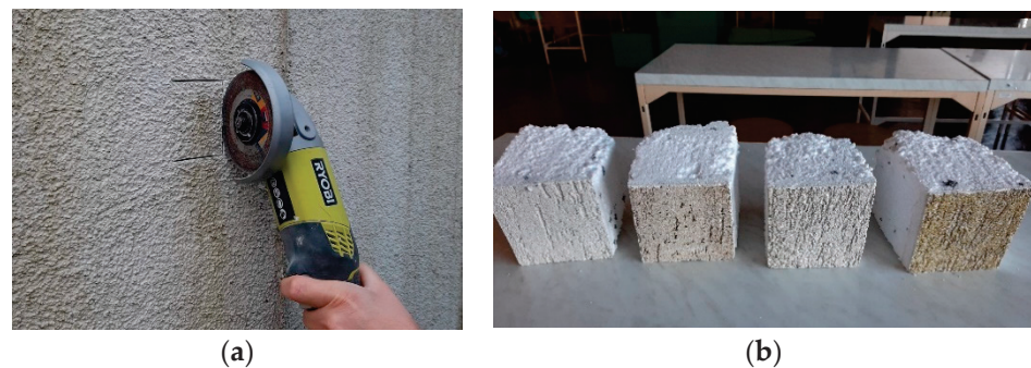
Figure 4. Sampling at the field site: (a) cutting the plaster surface; (b) samples that were cut out.
