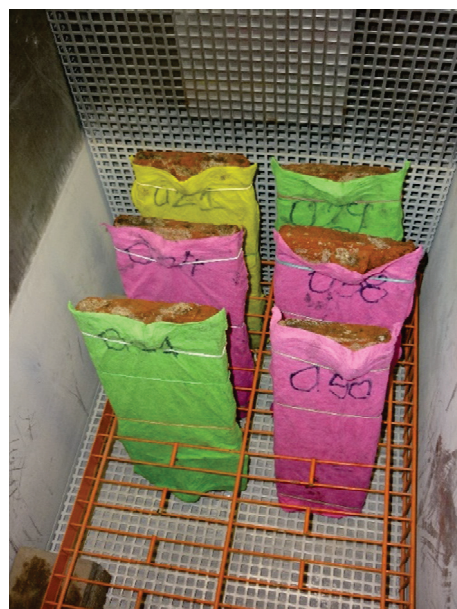
Figure 7. Roof tiles in a climate chamber.
