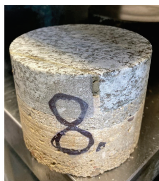
Figure 5. Core concrete sample No. 8 (borehole diameter 98 mm).
