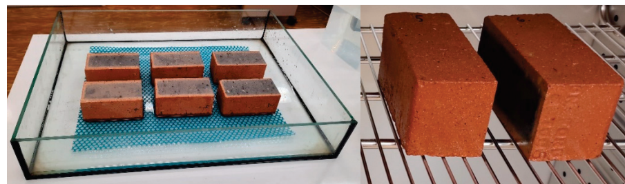
Figure 4. Sample conditioning in the authors' freeze–thaw durability method.
