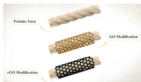
Figure 7. Images of the pristine, GO-modified, and rGO-modified CGYs [134].
