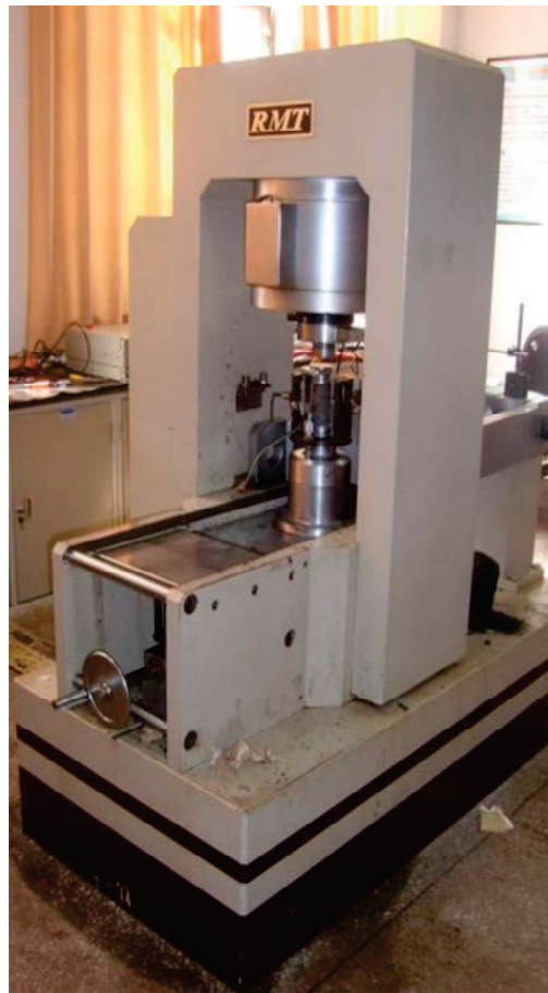
Figure 1. RMT-150-B electrohydraulic servo rock test system.
