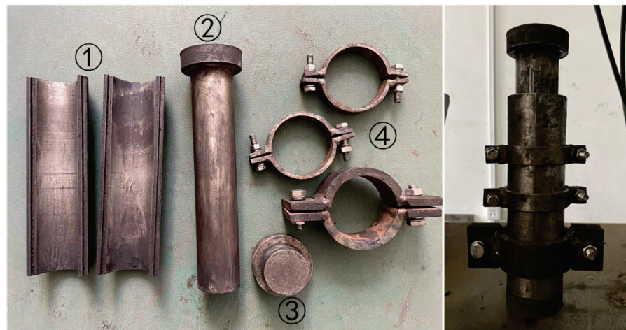
Figure 1. Specimen-producing mold. ① Semi-circular steel tube, ② compressive arm, ③ bottom plate, ④ fixing device.
