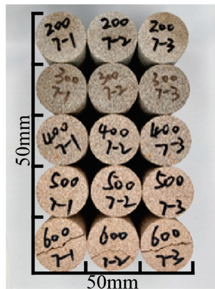
Figure 3. View of sandstone high-temperature water cooling.
