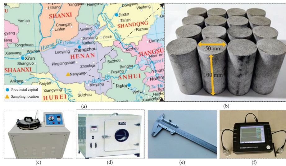
Figure 1. Sandstone sampling information and physical test equipment: (a) sampling location; (b) sandstone samples; (c) saturator; (d) dry oven; (e) saturation instrument; (f) acoustic test instrument.
