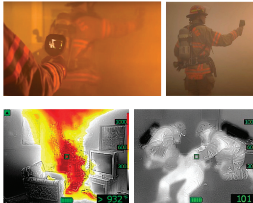
Figure 1. Images captured by thermal imaging cameras used by firefighters [6]. (From: https://www.flir.asia/discover/public-safety/no-excuse-for-firefighter-disorientation/ (accessed on 6 November 2022)).
