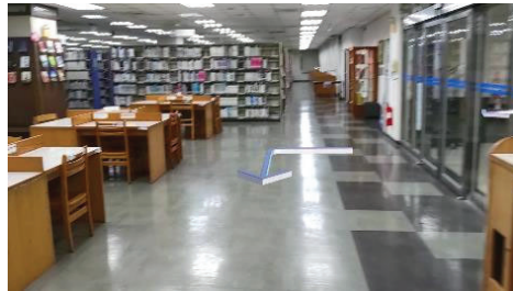
Figure 8. The positioned arrows will not disappear or move much, even after returning from long distance movement from the first anchor point.
