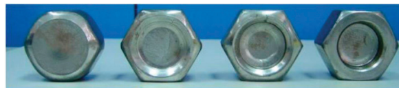
Figure 5. Actual stamped blank shape on-site.
