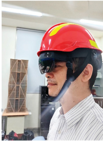
Figure 6. The WASS consists of a fire helmet and HoloLens 2, as well as other accessories.
