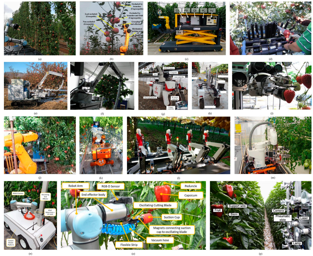
Figure 1. Typical harvesting robots. (a) A plum-harvesting robot (photo reprinted with permission from ref. [1]. 2021, Brown, J.); (b,d–f) Apple-harvesting robots (photo reprinted with permission from ref. [2]. 2021, Yan, B.; ref. [3]. 2017, He, L.; ref. [4]. 2012, Ji, W.; ref. [5]. 2011, Zhao, D.); (c,n–p) Sweet pepper-harvesting robots (photo reprinted with permission from ref. [6]. 2020, Arad, B.; ref. [7]. 2017, Lehnert, C.; ref. [8]. 2014, Bac, C.W.); (g–i) Strawberry-harvesting robots (photo reprinted with permission from ref. [9]. 2020, Xiong, Y.; ref. [10]. 2019, Xiong, Y.; ref. [11]. 2010, Hayashi, S.); (j) A lychee-harvesting robot (photo reprinted with permission from ref. [12]. 2018, Xiong, J.); (k,m) Tomato-harvesting robots (photo reprinted with permission from ref. [13]. 2018, Feng, Q.; ref. [14]. 2010, Kondo, N.); (l) A kiwifruit-harvesting robot (photo reprinted with permission from ref. [15]. 2019, Williams, H.A.M.).
