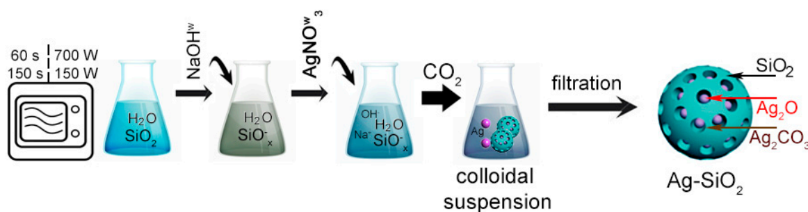
Figure 1. The synthesis of silver–silica spherical nanocomposites.
