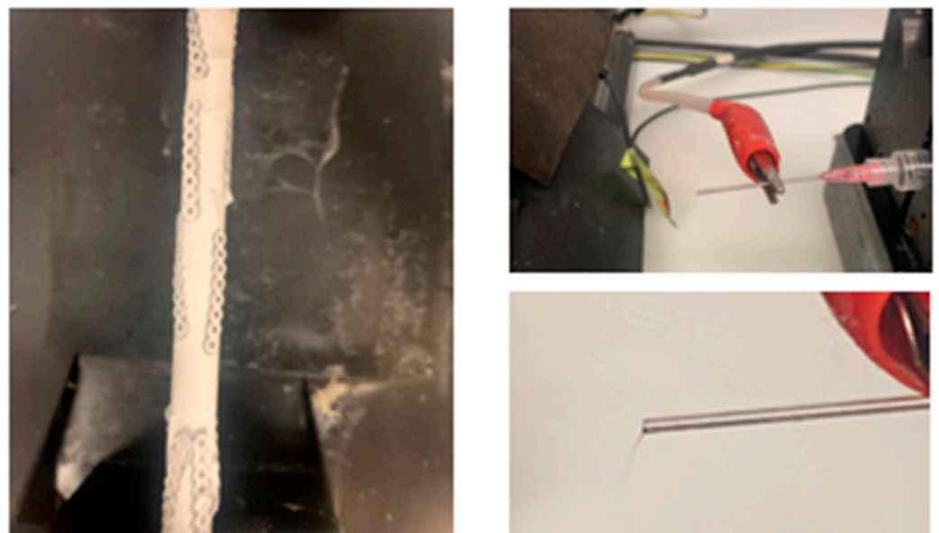
Figure 11. Photographs of the chains on the rotating rod ( left ) and polymer threads dispensing from the syringe ( right ).
