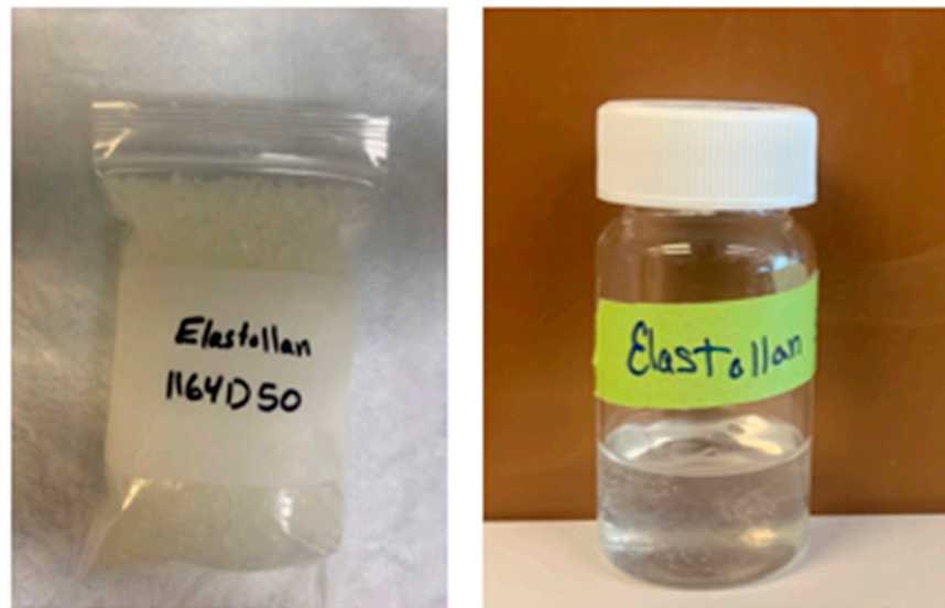
Figure 10. Elastollan ® polymer pellets ( left ) and final polymer solution ( right ).
