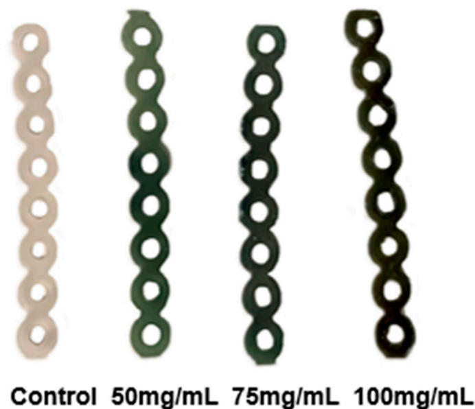
Figure 1. Experimental chains following SNAP impregnation demonstrating a light-to-dark gradient of green color.
