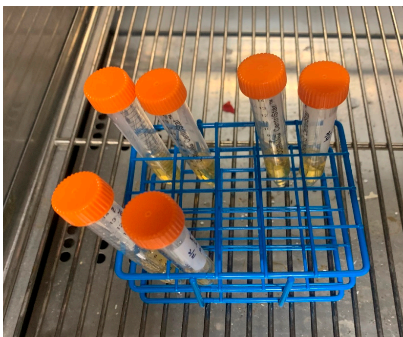
Figure 14. S. mutans in 4 mL solution of BHI + 2% sucrose. (Top left vials) control chains, (top right vials) chains impregnated with 75 mg/mL SNAP/THF, (bottom left) experimental chains (75 mg/mL SNAP/THF + Elastollan®).
