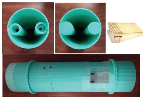
Figure 9. 3D printed sensor housing fabricated with PLA material in combination with PVA supportive material; the PT100 RTDs-integrated on PCB substrate are also presented (upper right image).
