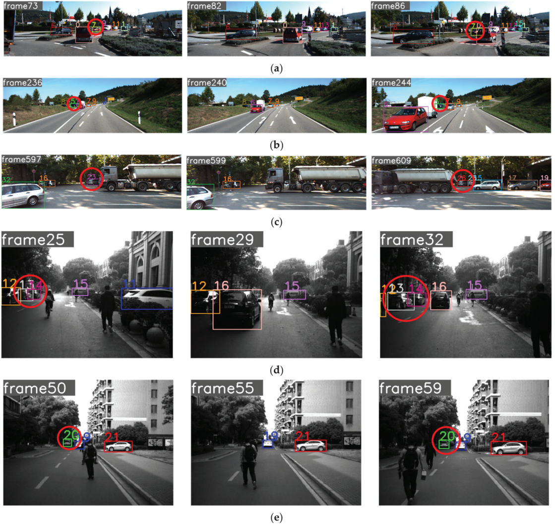
Figure 9. Tracking results. In each sequence, the tracked cars' IDs are located at the top of their bounding box, and the objects that will undergo severe or complete occlusion in subsequent frames are marked with red circles. (a) KITTI MOT testing-0008 tracking results. (b) KITTI MOT testing-0009 tracking results. (c) KITTI MOT testing-0015 tracking results. (d) Real-world campus scenarios-0001 tracking results. (e) Real-world campus scenarios-0003 tracking results.
