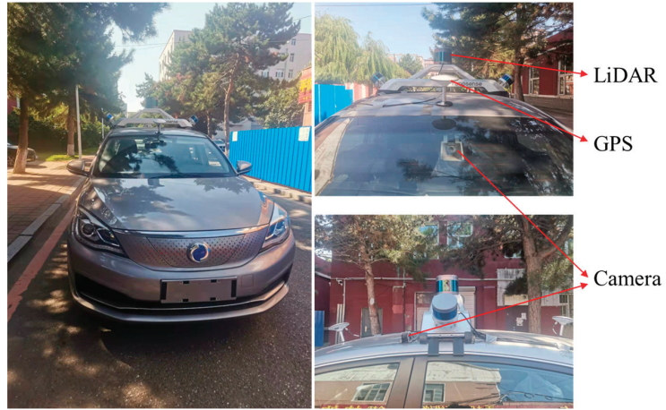
Figure 19. Vehicle for recording mapping data, equipped with RTK-GPS, LiDAR, and cameras.
