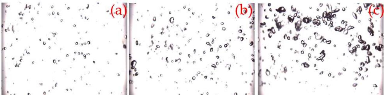
**Figure 6.** Distribution of bubbles with different air contents: (a) 0.05 air content; (b) 0.1 air content; (c) 0.15 air content.
