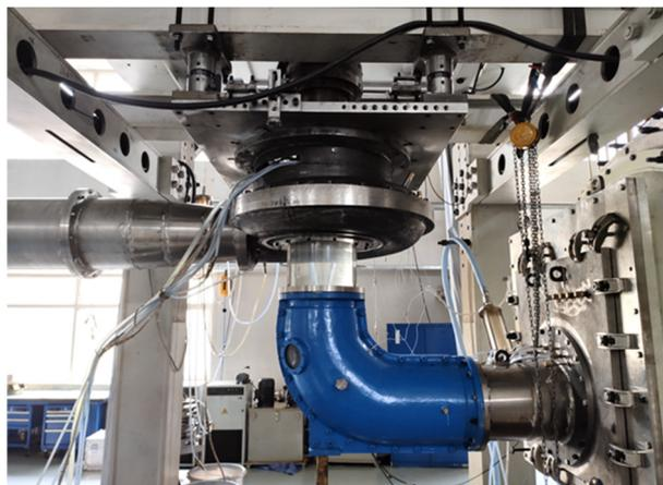
**Figure 9.** Centrifugal pump model test rig.
