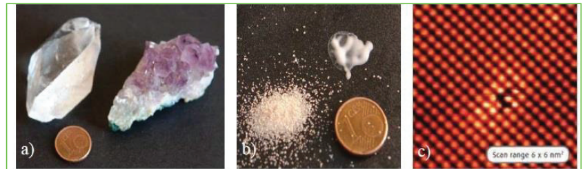
Figure 12. Hyper-constructivist tex-book (not “textbook”) [51]: touching the dimensions of an atom, by dividing the crystal of quartz (a); into sand by one thousand times (b), and again by one thousand times ((b), upper right corner) into a polishing liquid. Photo (c): picture of silicon crystal seen by atomic force microscope, 6 \times 6 \text{ nm}^2 , Omicron. Text and photo GK. Reproduced from ref. [51] with permission.
