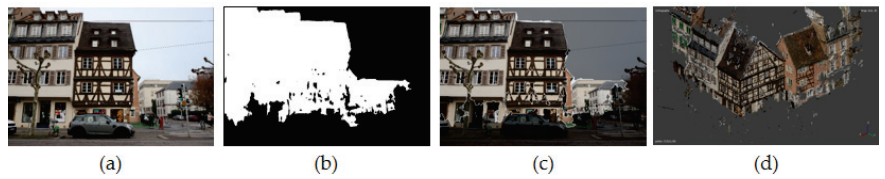
Figure 7. Example of concrete application of the proposed method in photogrammetric point cloud cleaning: (a) original image, (b) mask of all classes except “background”, (c) mask applied to the original image and (d) 3D point cloud from dense image matching using the masked image.
