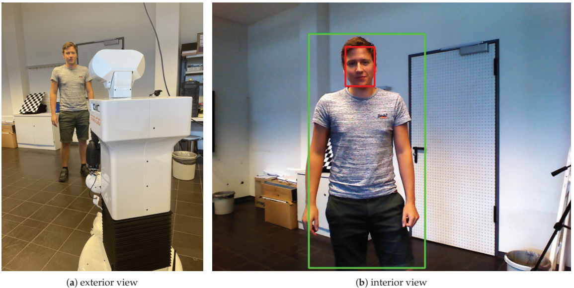
Figure 5. Our proposed SFPD network implemented on a mobile robot system for human–robot interaction in a demo application: (a) exterior view and (b) interior view of the robot.
