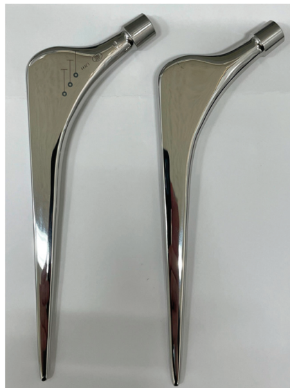
Figure 1. Exeter stem (SUS) and Exeter-shaped CoCr stem. On the left is an original Exeter stem. On the right is our Exeter-shaped stem of CoCr. The Exeter-shaped CoCr stem was made using the exact same design and surface roughness as the original stem.
