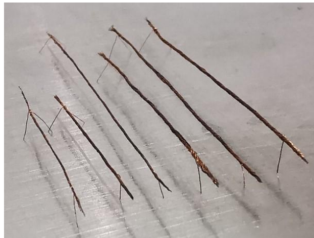
Figure 15. Different masses of manufactured beam-shaped copper wire weights.
