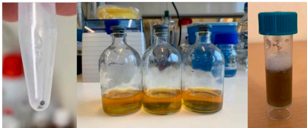
Figure 3. Pellet of the centrifuged sample (left), samples prepared for lyophilization (middle) and sample after solvent elimination by evaporation (right).
