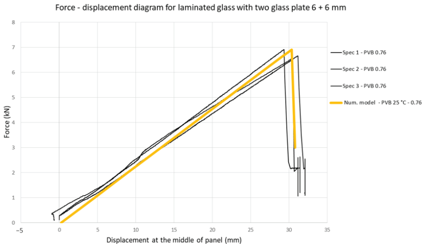
Figure 7. Force-displacement diagram: results of four-point bending from the numerical and experimental tests.
