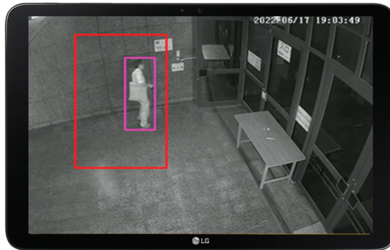
Figure 1. FenceTalk user GUI. (Red polygon: fenced region; Pink square: the moving object).
