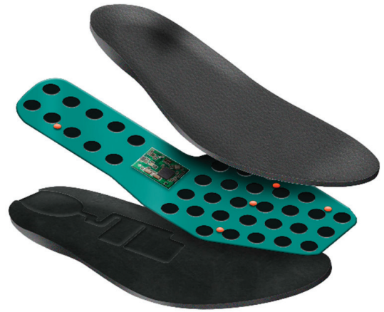
Figure 2. Insole sensory regions. (A) Pressure-sensing regions. (B) Temperature-sensing regions. (C) Multimodal sensory insole system containing pressure, temperature, and motion sensors embedded in a custom orthotic. Large black circles illustrate the array of discrete force sensitive resistors (FSR) to record plantar pressure. Small orange circles illustrate the five temperature sensors located beneath the high-risk bony prominences in the foot (metatarsal heads 1, 3, and 5, the heel, and the big toe). At the time of the study, temperature asymmetry monitoring was inactive at the big toe. The inertial measurement unit (IMU) is embedded in the electronics chip in the center of the insole.
