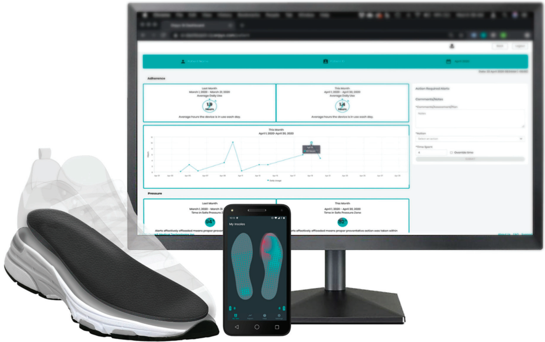
Figure 1. The Sensory Insole System (Orpyx ® Sensory Insole System, Orpyx Medical Technologies Inc., Calgary, AB, Canada) includes custom-milled insoles that are placed into the patient’s shoes; a patient-facing app that provides real-time pressure feedback, step count, and wear time information; and a web-based dashboard accessed by a remote patient monitoring nurse and provider to review the data collected from the sensory insoles.
