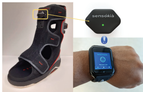
Figure 3. The overall smart offloading system, used by participants assigned to use the smart removable cast walker (sRCW). The system consists of a sensor that attaches to the cast walker, as well as a watch that provides the participant notifications regarding their adherence.
