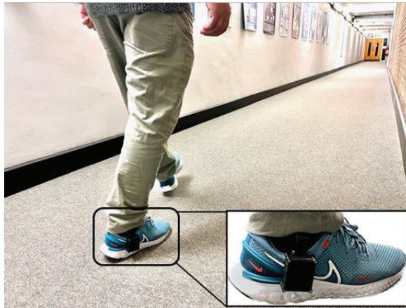
Figure 6. A photo showing level walking along a 28 m indoor corridor with the device attached to the footwear.
