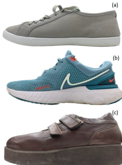
Figure 7. (a) Plimsoll with a flat sole, (b) trainer as a standard type of footwear used in the experiment and (c) therapeutic footwear with rocker features.
