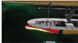
Figure 5. Initial state of the ship model test with fixed model attitude.
