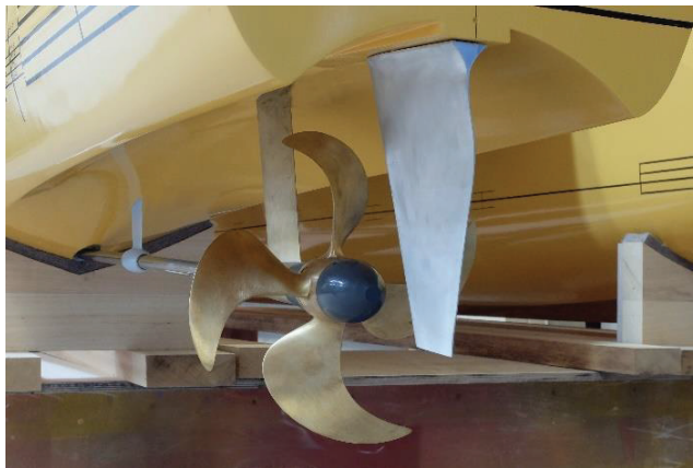
Figure 15. Close-up of the stern area of the tested Stavanger model, with fitted propellers, shafts, brackets and rudders.
