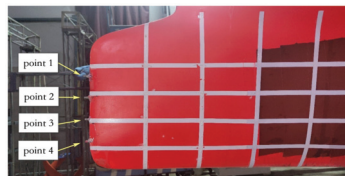
Figure 6. Schematic diagram of the bubble generation location.
