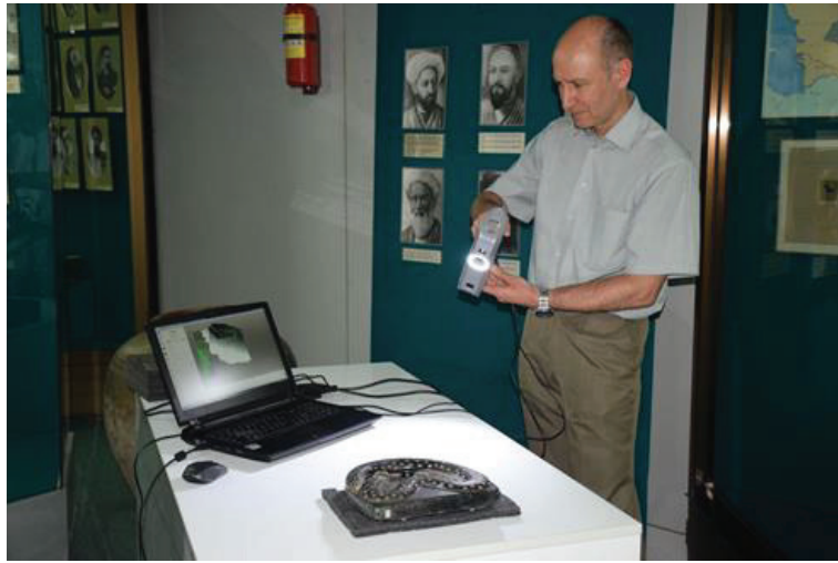
Figure 3. Scanning environment arrangement to scan the “Snake” figure.
