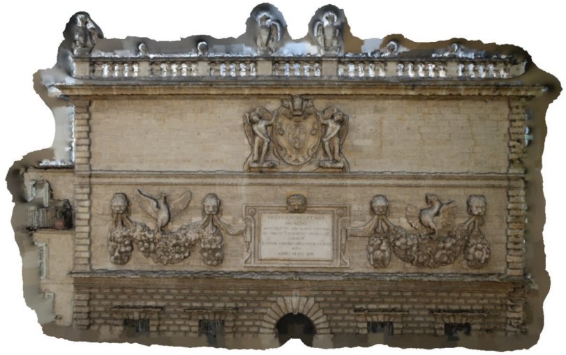
Figure 14. Texture model of the Hotel sequence that was reconstructed by the Poisson surface reconstruction. The textured model has a high geometry consistency with the real scene.
