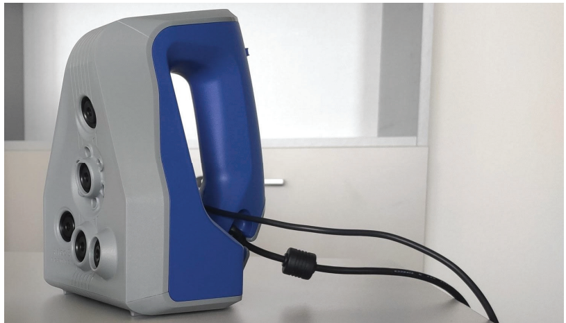
Figure 3. Artec 3D Space Spider structured-light scanner.
