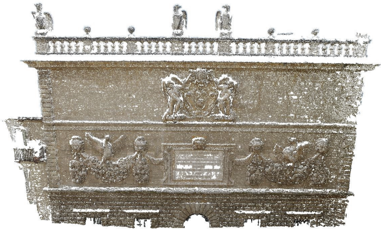
Figure 13. MVS data of the Hotel sequence that was generated by the PMVS. The dense point clouds are very accurate. This is attributed to use of the HashMatch method.
