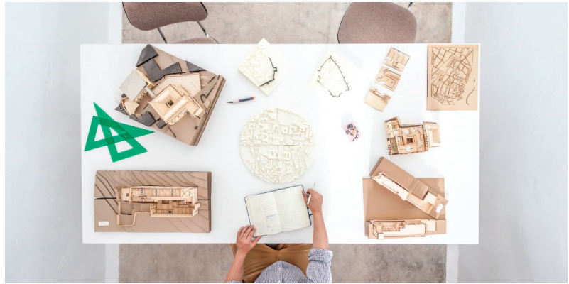
Figure 5. Different examples of physical models of architecture obtained using different 3D printing and cutting systems. TAD3 Lab. Works in collaboration between the University of the Americas of Puebla and the University of Extremadura. In the figure, we can see models made of wood on both sides that have been executed with a laser printer and CNC cutting machine, and, in the center of the table, we can see white filament models that have been manufactured with a filament extrusion printing printer.
