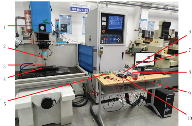
Figure 11. Experimental system of micro-EDM. 1: Micro electrical discharge machining. 2: Magnetic actuator. 3: Tool electrode. 4: Machining workpiece. 5: Discharge gap voltage detection circuit. 6: Switching DC power supply. 7: Computer. 8: dSPACE1104. 9: Multimeter. 10: Current power amplifier.
