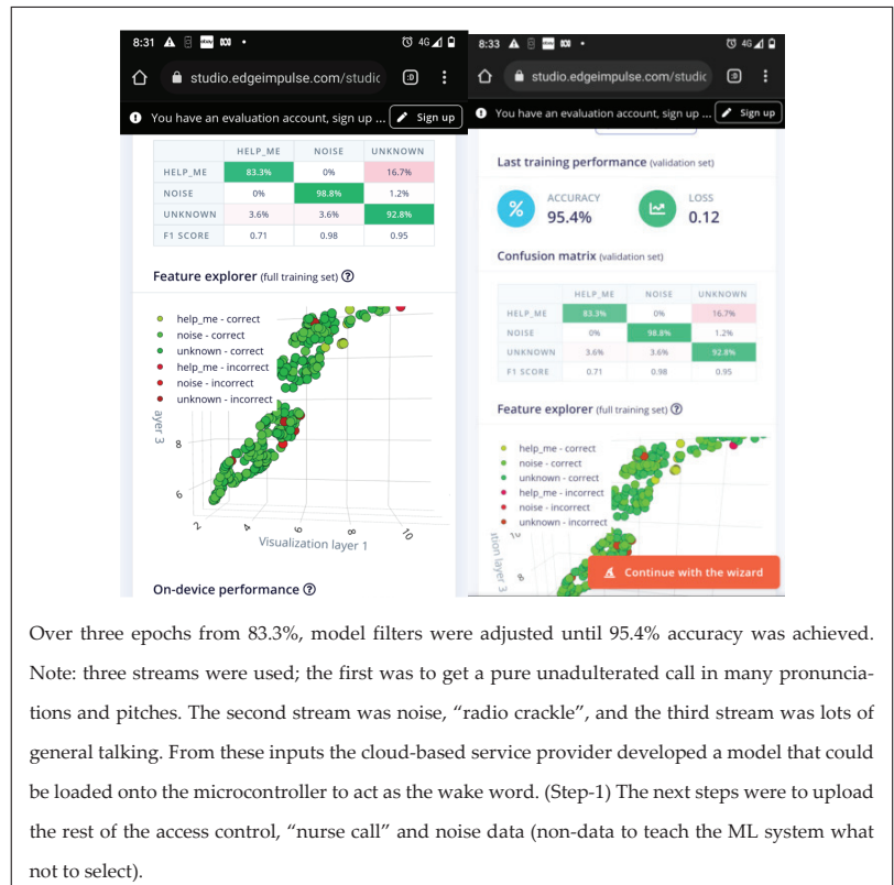
Figure 16. “Wake word” planning, configuration, tests and results.
