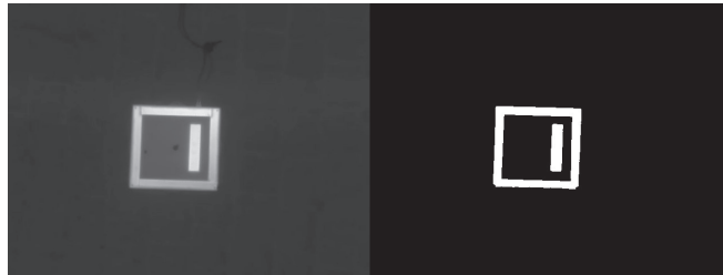
Figure 2. The binary threshold operation applied to the infrared images.
