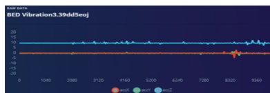
Figure 18. Bed vibration with fixed sensor.
