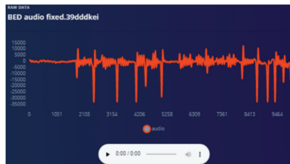
Figure 21. Response from audio when sensor fixed to a hard surface.
