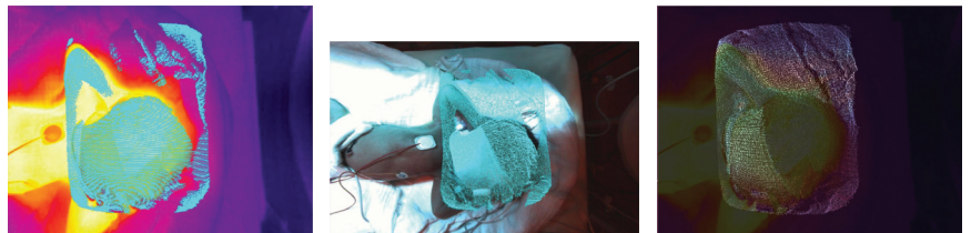
Figure 11. Thermal-ToF-fusion (left), RGB-ToF fusion (middle) and thermal-RGB-fusion camera image (right).
