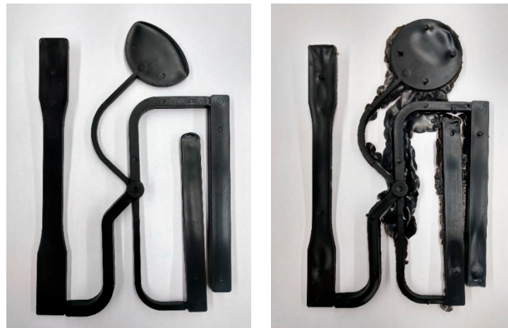
Figure 2. Examples of defect types: short shot, flash, and sink marks.
