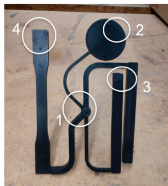
Figure 8. Visual quality standard zones (labeled 1–4) on molded parts.
