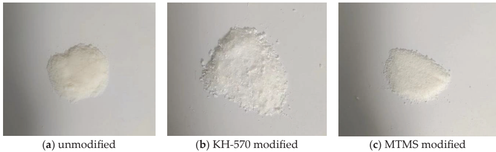
Figure 12. Diagram of different reinforced modified silica aerogel.
