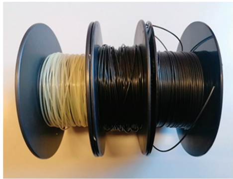
Figure 4. 3D printing filaments obtained from extrusion processing.
