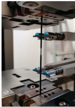
Figure 6. Tensile test of a filament.
