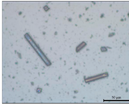
Figure 9. Carbon microfibers under the optical microscope (magnification 50 \times ).
