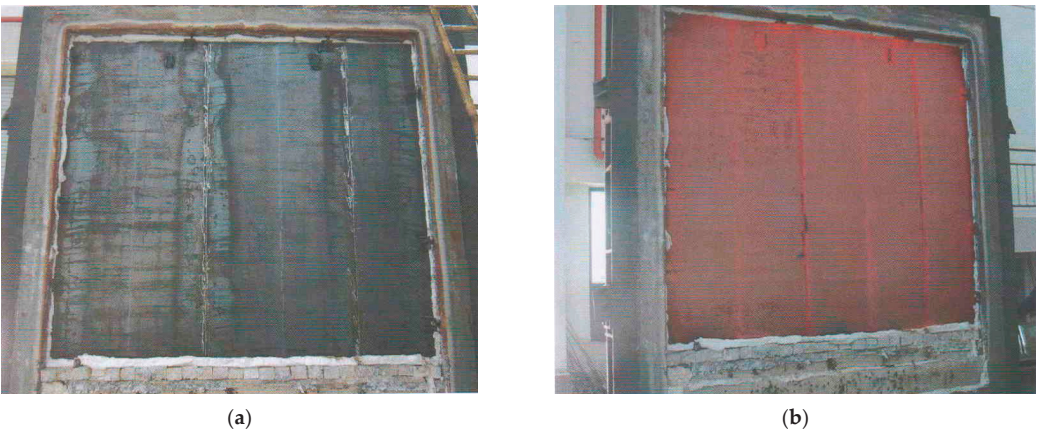
Figure 7. Heated surface of the A-60 bulkhead before (a) and after (b) fire test (60 min).
