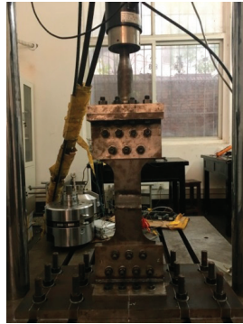
Figure 2. Scheme of fatigue crack growth test.
