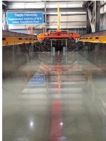
Figure 21. Installation of displacement transducers.
