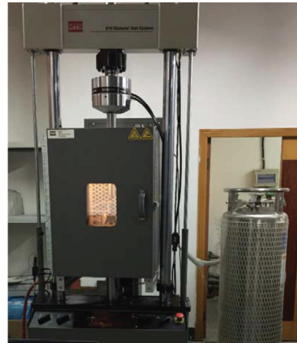
(b) Experimental setup for low strain rate tensile tests.
