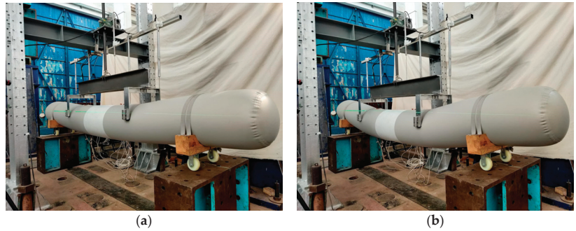
Figure 10. Deflected process of the inflated sample: (a) initial loading; (b) close to ultimate load.
