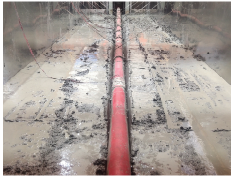
Figure 35. Developed trench shape.
