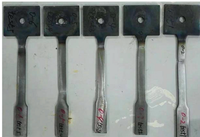
Figure 3. Failure of the quasi-static test specimen.
