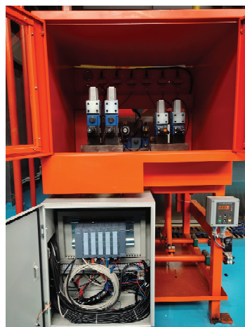
Figure 11. Assembly of the electrohydraulic servo valves and electrical control cabinet.
