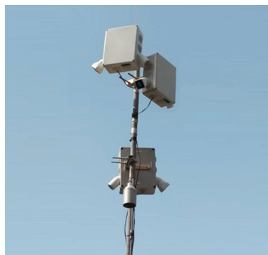
Figure 4. Picture of the three sensor nodes of the air quality monitoring system developed.
