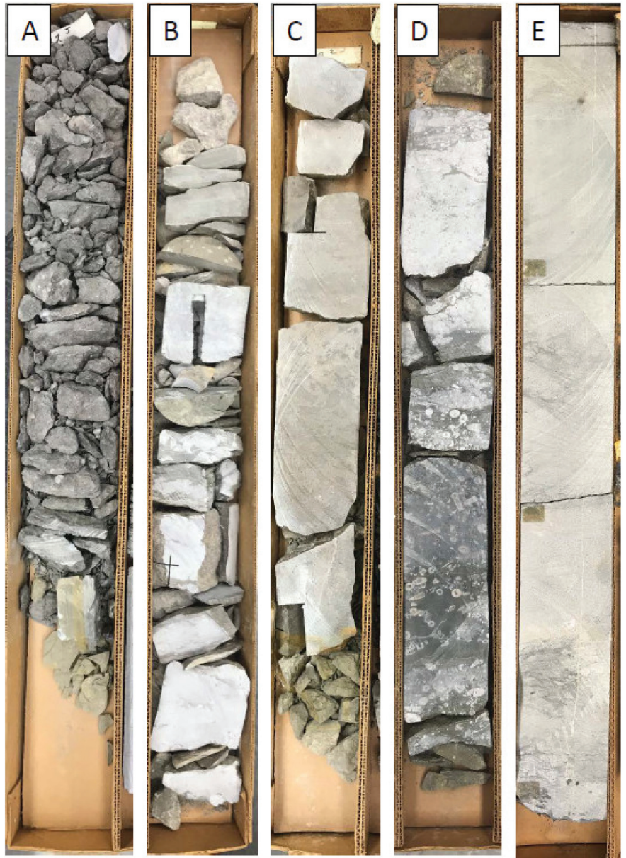
Figure 3. Examples showing variations in core integrity. (A) rubble, (B) rubble with intact sections, (C) partially intact, (D) mostly intact, (E) completely intact. Core intervals with missing pieces or being broken does not impact the core integrity call.
