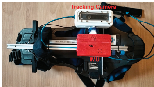
Figure 2. Sensor assembly mounted on the firefighter equipment.
