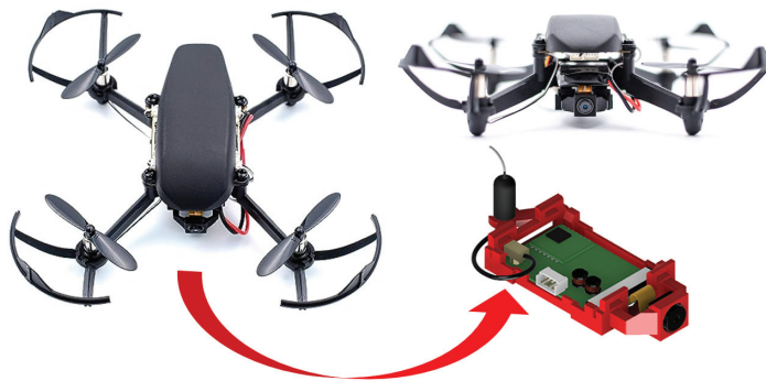
Figure 4. Drone with WiFi Camera Module.
