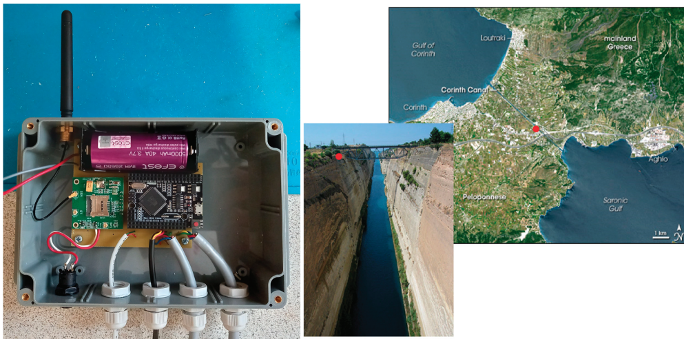
Figure 2. A photograph of the complete prototype (left) and the first deployment location (right). The red dot shows the exact location of the first system deployment.
