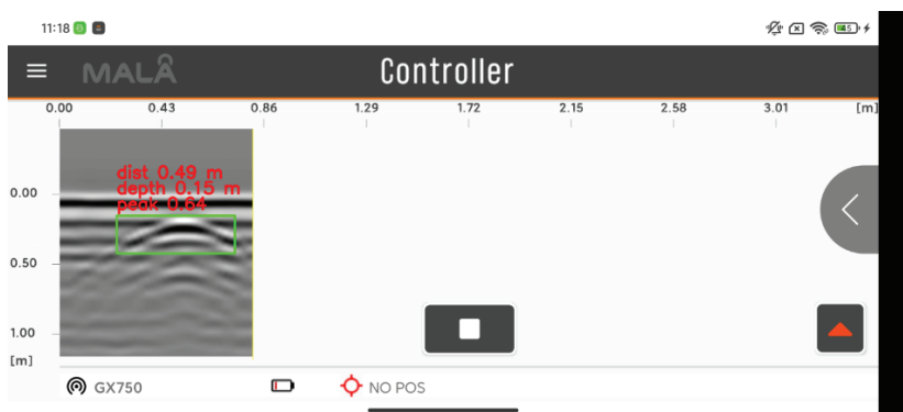
(a) The result of the real-time detection system used to identify the ground-penetrating radar results after passing over the first steel bar.
