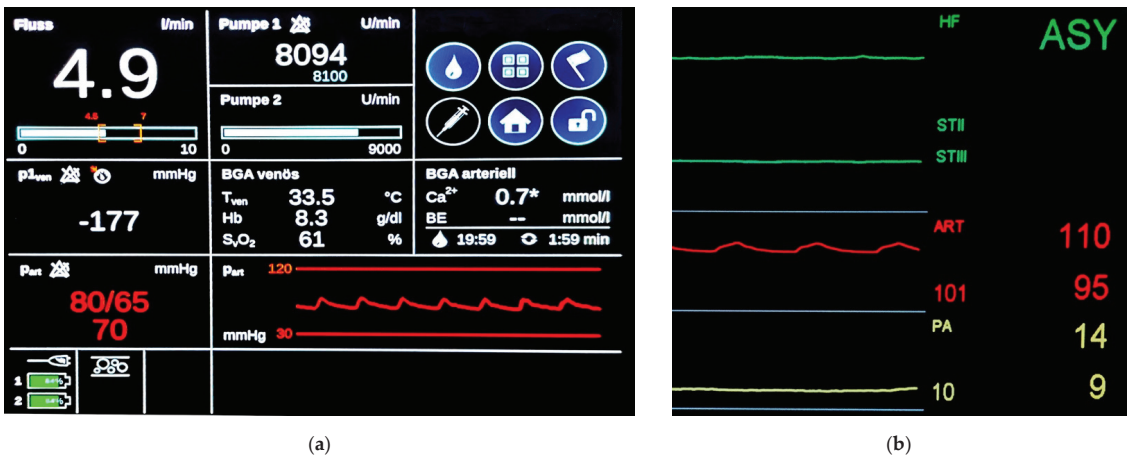
Figure 2. Pulsatile blood flow on ECC during CARL therapy: (a) Screenshot from real-time measurements on the CARL controller during asystole reperfusion. A pulsatile blood pressure was observed during extracorporeal circulation in the ascending aorta during asystole phase (red curve); (b) Screenshot of experimental monitoring during ECC. Despite asystole (green curve), a pulsatile blood flow (red curve) is detected in the common carotid. Pulmonary artery (PA) pressure is displayed in yellow.
