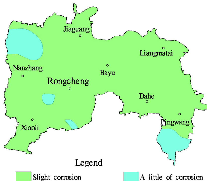
Figure 8. Zonal distributions of chemical corrosion of steel by groundwater.
