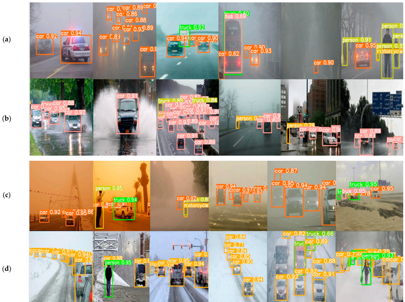
Figure 9. Vehicle detection results on the DAWN dataset row-wise: (a) fog; (b) rain; (c) sand; and (d) snow.
