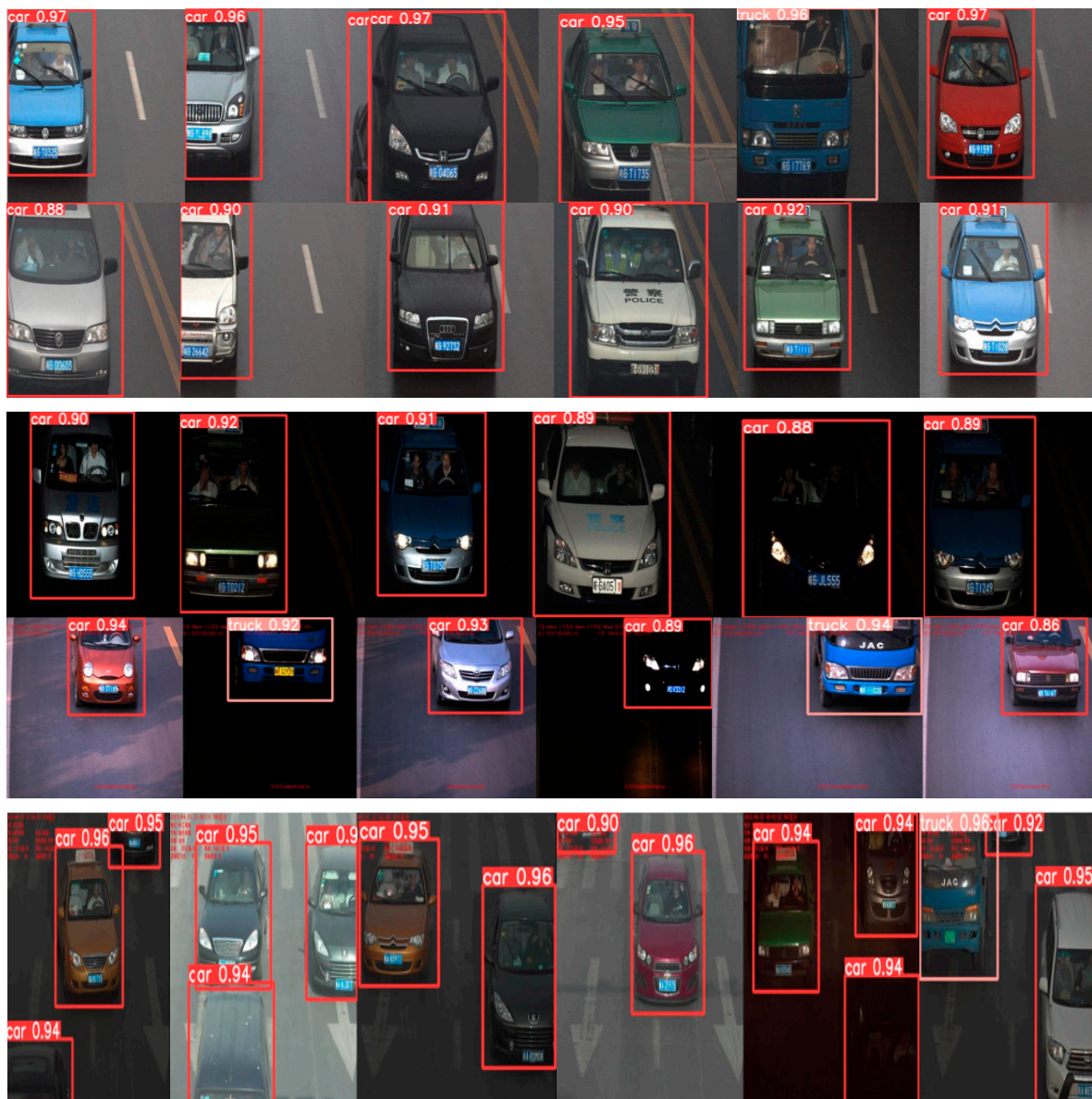
Figure 7. Vehicle detection results on the PKU dataset from G1 to G5 categories
