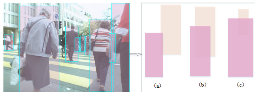
Figure 6. Target occlusion diagram: (a) similarly proportioned pedestrian non-influential screening; (b) similarly proportioned pedestrian-impacted screening; (c) disparately proportioned pedestrian-impacted screening.
