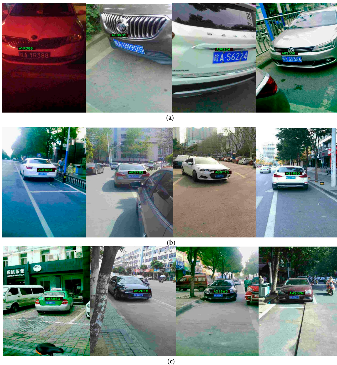
Figure 7. The LPR on the CCPD dataset for (a) base, (b) blur, and (c) FN scenarios.
