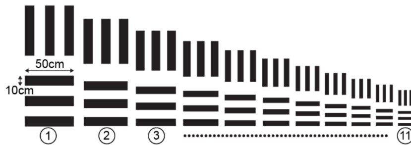
Figure 7. Specification of simple resolution bar target for UAV photogrammetry.
