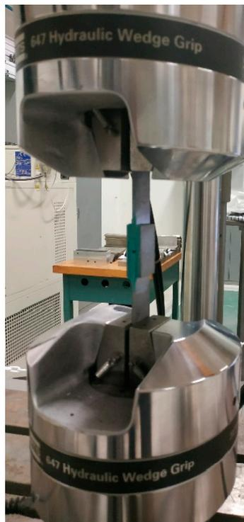
**Figure 5.** Experimental set-up of double lap shear tests.
