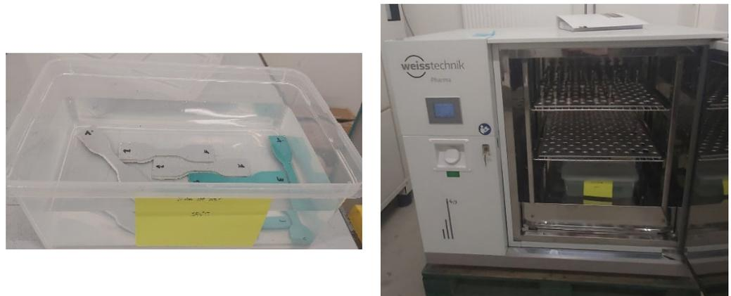
**Figure 4.** Testing container (on the (left)) and climate chamber/oven (on the (right)).
