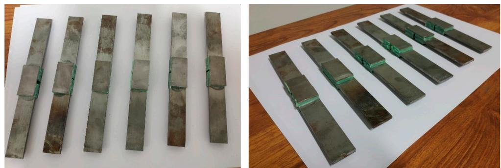
Figure 3. Double lap shear adhesive specimens.
