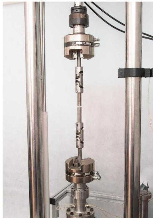
**Figure 3.** The adhesive specimen in the jointed fixture of the testing machine.
