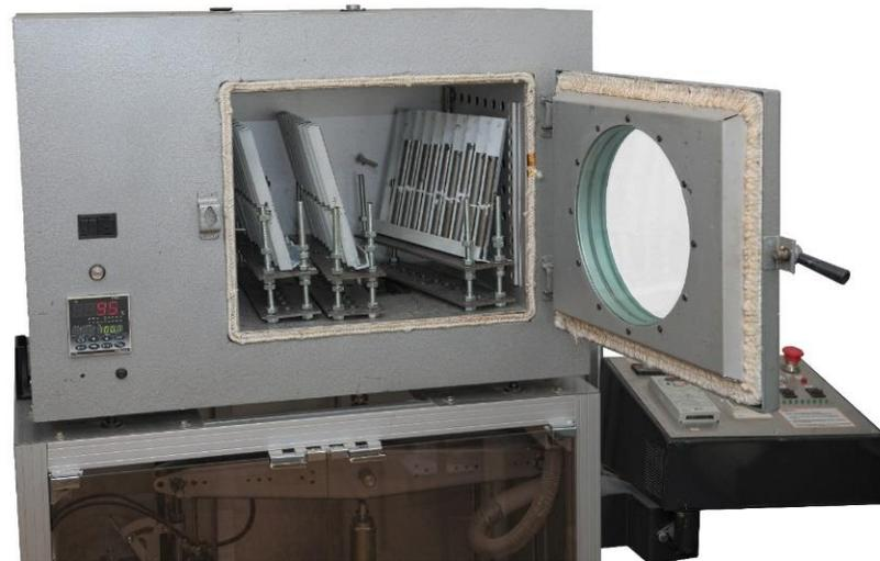
**Figure 2.** Positioning brackets for the correct orientation of the bonded specimens in the heating chamber.
