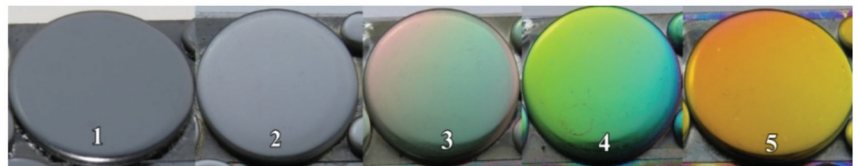
Figure 10. The perceived colour of the TaTiON coatings: 1—Ta1–Ti0–ON; 2—Ta0.75–Ti0.25–ON; 3—Ta0.5–Ti0.5–ON; 4—Ta0.25–Ti0.75–ON; 5—Ta0–Ti1–ON.
