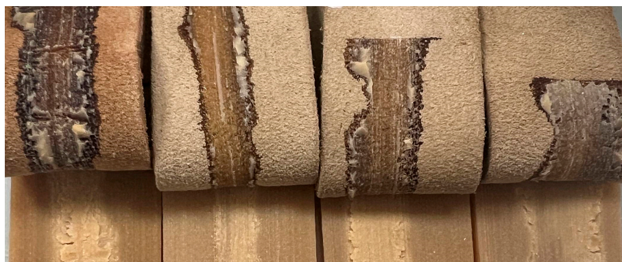
Figure 12. Appearance of samples after T-peel test. From left to right: HMPUR-REF, LIGNOC-2.5%, LIGNOC-5%, and LIGNOC-7.5%.
