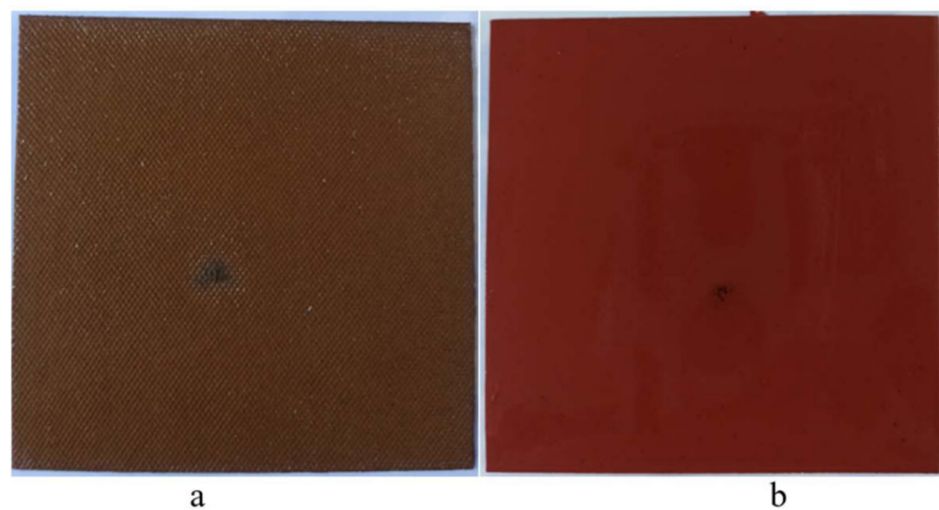
Figure 2. Surface breakdown points at 25.2 kV ((a) pressboard and (b) polyurethane).
