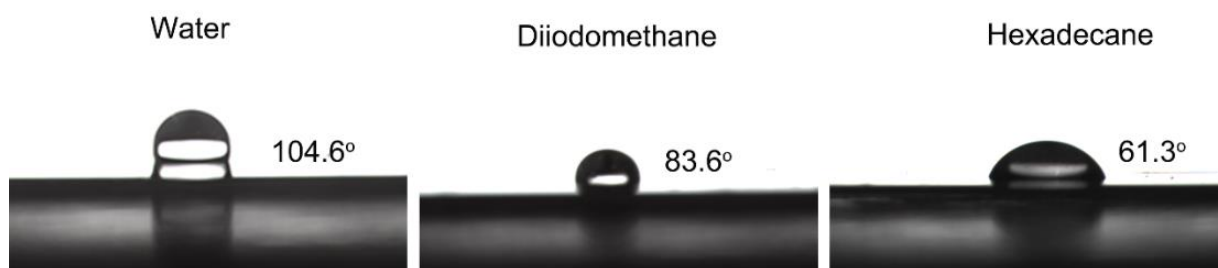
Figure 7. Images of droplets and the contact angles of water, diiodomethane, and hexadecane on the coating.
