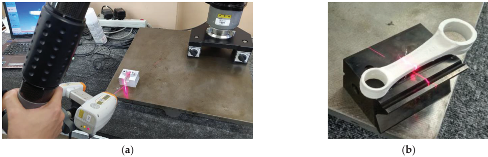
Figure 2. Measurement using a laser scanner of: (a) a model for clamping and positioning parts in a machining process; (b) a connecting rod.
