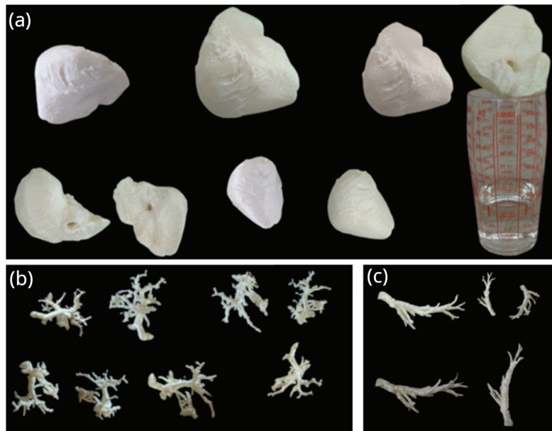
Figure 2. (a) 3D-printed liver mold (145 mL of internal volume); (b) 3D-printed liver vein mold; (c) 3D printed liver artery mold.
