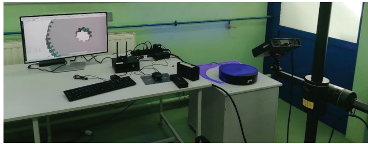
Figure 3. Measurement stand equipped with a structured light scanner.
