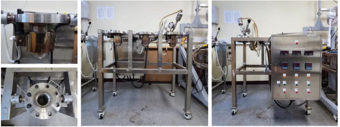
Figure 1. Laboratory-scale hydrothermal carbonization reactor (0.2 L).
