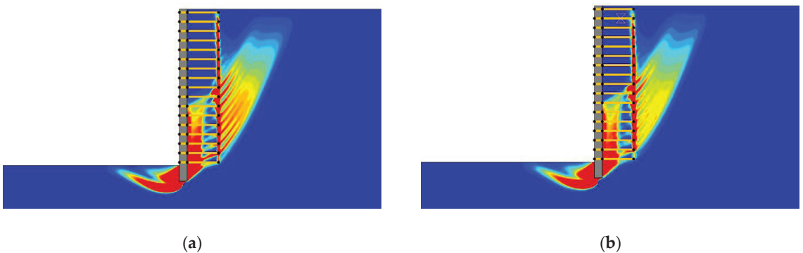
Figure 1. Comparison of the different numbers of elements. (a) Safety factor = 0.8752 (elements = 10,000). (b) Safety factor = 0.8781 (elements = 20,000).
