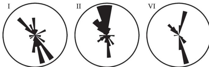
Figure 6. Rose diagrams of nodal strikes for focal mechanism in three regions of Baihetan Reservoir.
