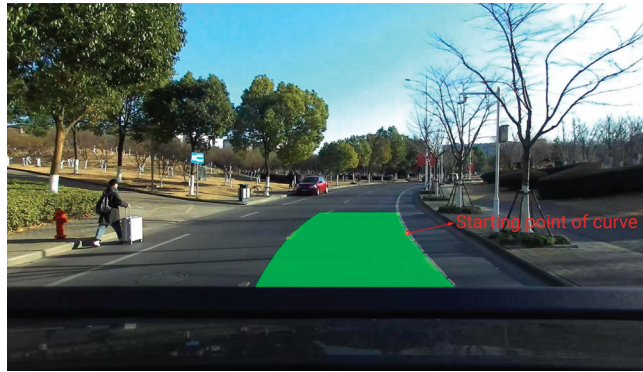
Figure 12. Lane-line circle-curve starting-point detection.
