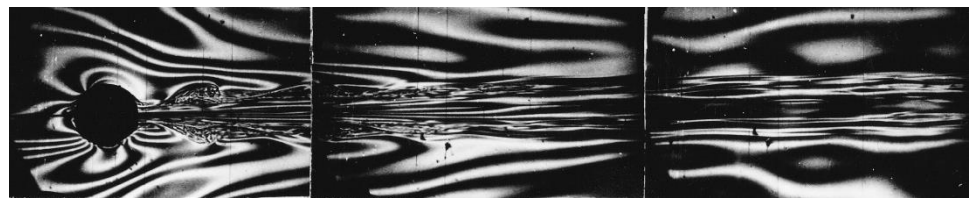
Figure 16. Black and white replica of the color schlieren image of the flow in the wake of the sphere: T_b = 3.0 s, N = 2.09 s ^{-1} , D = 4 cm, U = 1.45 cm/s, Re = 780 , Fr = 0.03 .
