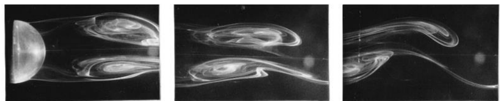
Figure 13. Evolution of an electrolytic precipitation suspension pattern in the wake past a sphere in CSF (top view): T_b = 8.0 s, N = 0.785 s ^{-1} , D = 5 cm, U = 0.65 cm/s, Re = 325 ; Fr = 0.027 ; time interval between frames \Delta t = 1 s.
