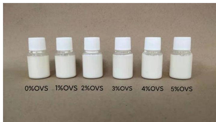
Figure 2. The appearance state of the OVS modified emulsion after 90 days of placement.
