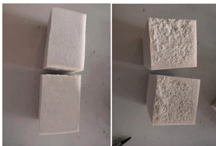
Figure 9. Tensile fracture cross-sectional morphology of unmodified neoprene latex specimens (fracture at the sample bond).
