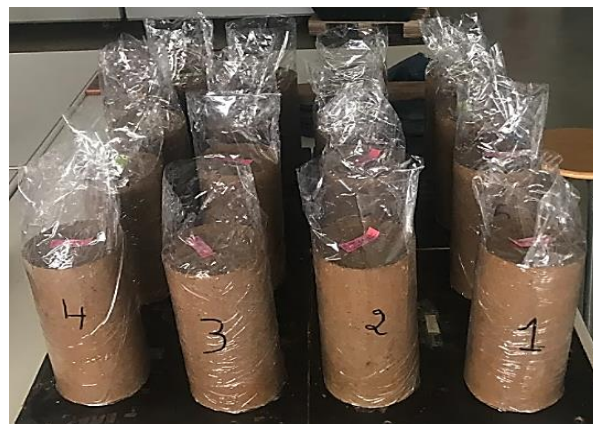
Figure 3. Samples coverage to homogenize water content (the samples are numbered from 1 to 24).
