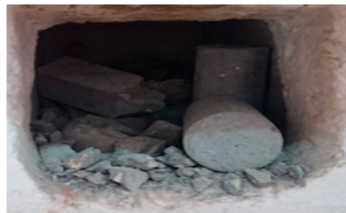
Figure 17. When SCC with and without glass fibers samples are heated to 450 °C, explosive spalling ensues.
