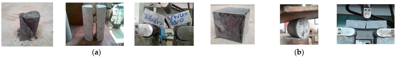
Figure 15. Failure patterns of SCC samples. (a) Specimens without fibers. (b) Specimens with fibers.
