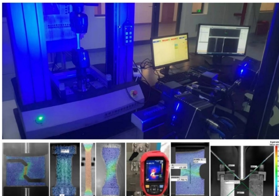
Figure 2. Universal mechanical experimental machine and XTOP digital image correlation system.
