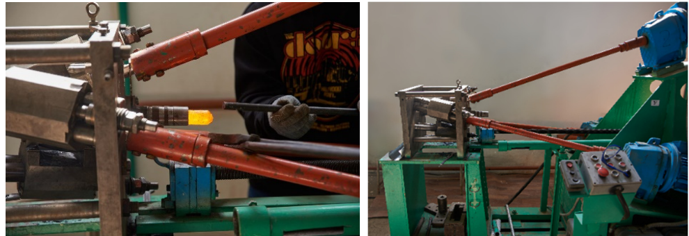
Figure 4. Experimental rolling and the RSR-10/30 radial shear rolling mill.
