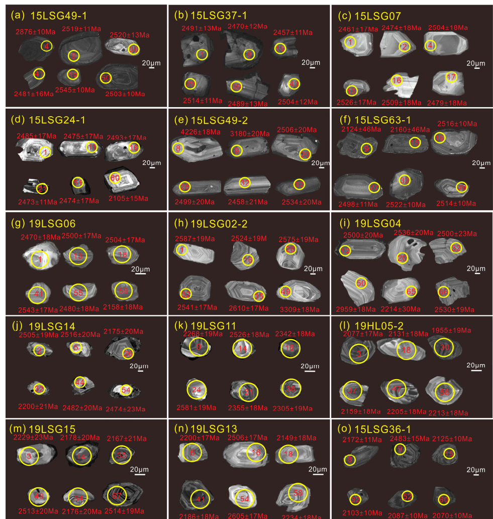
Figure 6. (a–c) Representative CL images of zircon from sedimentary rocks in Lower Langzishan Fm., (d–k) representative CL images of zircon from sedimentary rocks in Upper Langzishan Fm., (l–o) representative CL images of zircon from sedimentary rocks in Li’eryu Fm. Yellow circles indicate the experimental positions.
